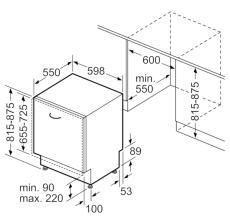
measurements in mm
